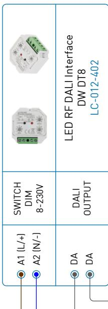
The number of scenes that can be used depends on the control panel, the remote control has a max. 6 pieces and the app is max. 8 pieces. If the rotary switch on the DALI RF interface at Scene position "1" to "15" the DALI groups 0-14 are addressed directly, with the setting "1" then the DALI group 0 corresponds to and "15" of the DALI group 14.
