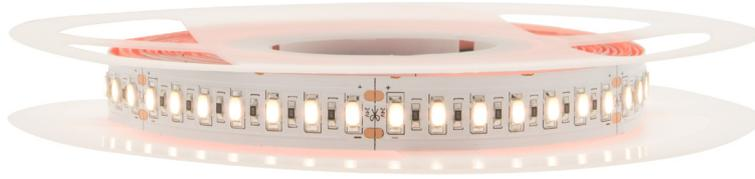
5m per reel LED Flexstrip 150 with 50cm long connection cable at the beginning and the end, each with 0.75mm<sup>2</sup> cable cross-section. Each package includes one 10cm long piece of heat shrink tubing with hot melt glue by heating up that can be used after cutting at the beginning and at the end. Due to its high wattage performance and the associated heat dissipation development, this LED strip does not covered a shrink tubing jacket and therefore no increased degree of protection!
