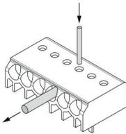
Loosen wire through twisting and pulling or using a 1 mm diameter release tool
